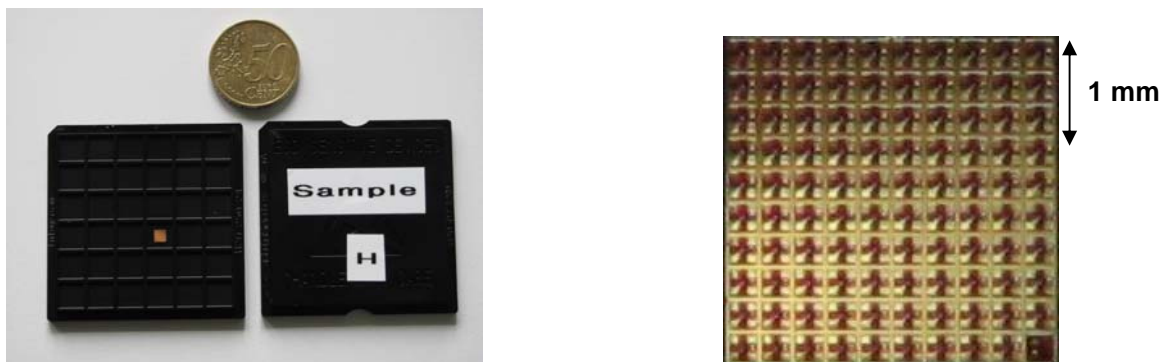
Figure 1: Photograph of the flip-chip bondable VCSEL sample in a chip carrier (left) and zoomed view (right).
