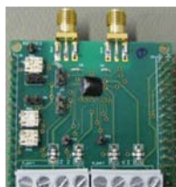
RF test board with bonded ASIC
