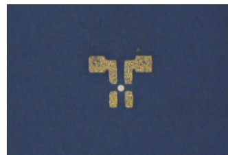
Anti's manufactured LTCC platform pads for pads of VCSEL (VTT)
